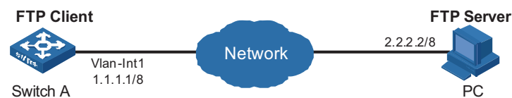
Figure 150 Network diagram for FTP configurations: a switch operating as an FTP client
