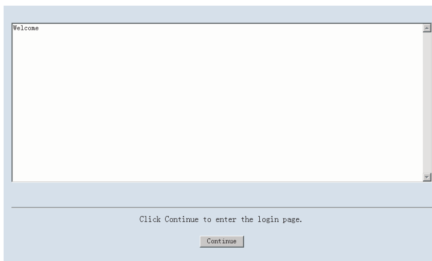
Figure 24 Banner page displayed when a user logs in to the switch through Web
