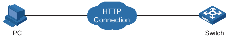
Figure 21 Establish an HTTP connection between your PC and the switch
