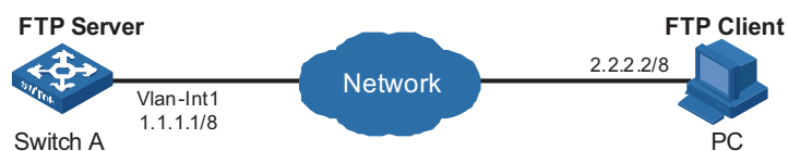
Figure 148 Network diagram for FTP configurations: a switch operating as an FTP server
