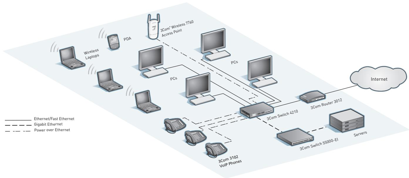
In the above network, 3Com Switch 4210 and Switch 5500G-EI units are managed as a single cluster.
