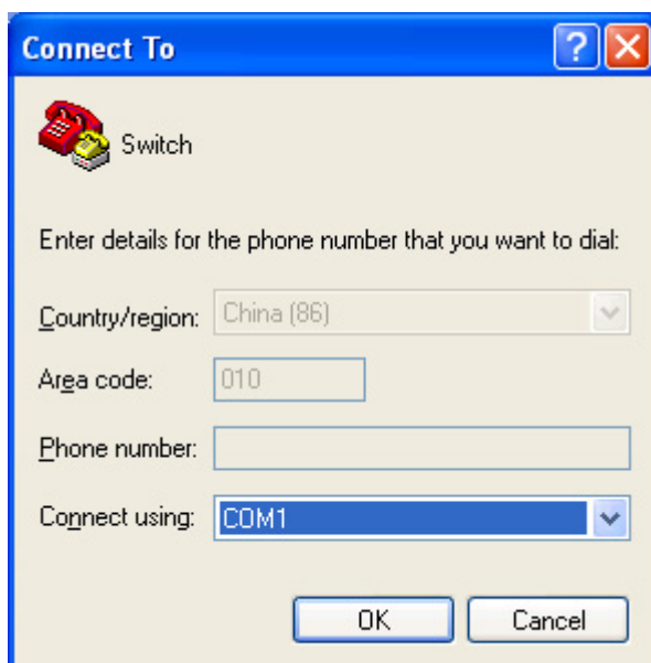
Figure 4-3 Set serial port for HyperTerminal connection
