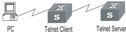
Figure 7 Provide Telnet Client service
