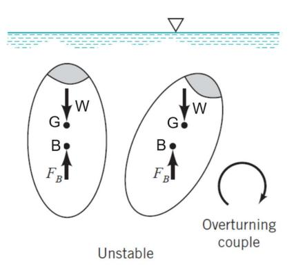
Stability of a completely immersed Body - center of gravity above centroid.
