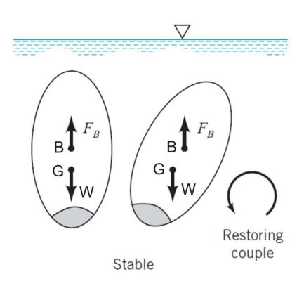
Stability of a completely immersed body - center of gravity below centroid.
