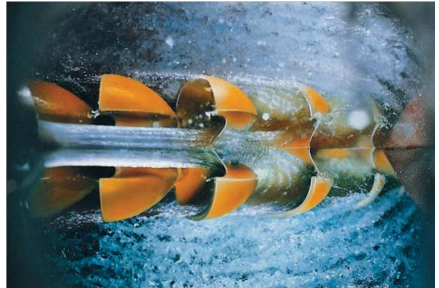
A view from the bottom of an operating Pelton wheel
