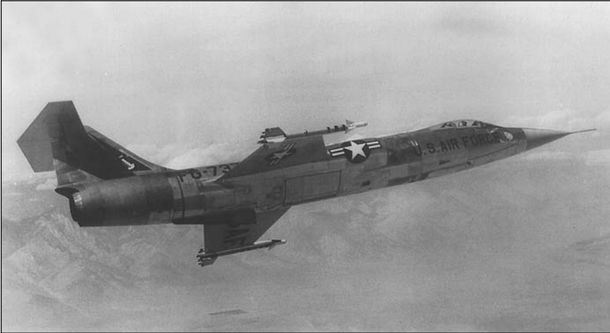
Figure 5.40 The first airplane to be designed for sustained flight at Mach 2: the Lockheed F-104 Starfighter.
