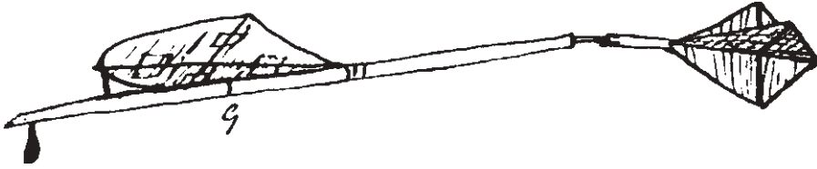
Figure 1.8 The first modern-configuration airplane in history: Cayley’s model glider, 1804.
