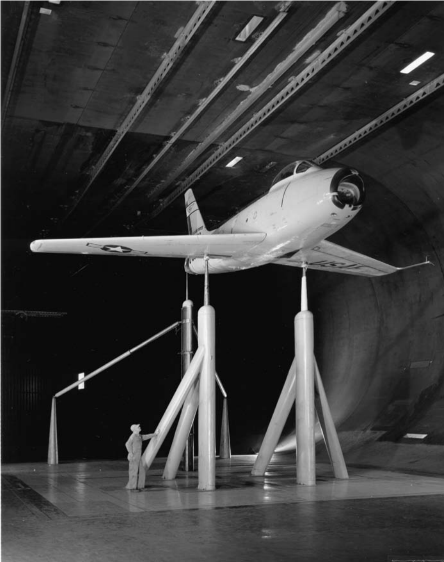
Figure 4.60 A subsonic wind tunnel large enough to test a full-size airplane. The NASA Langley Research Center 30 ft \times 60 ft tunnel. (Source: NASA.)
