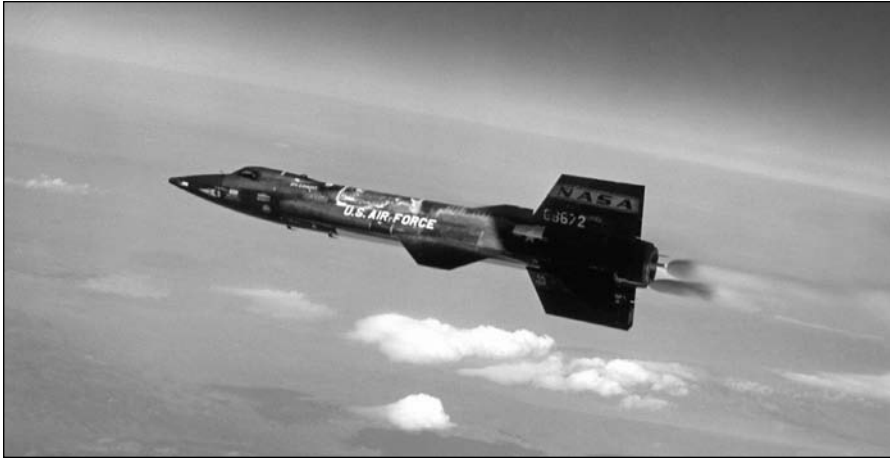
Figure 5.92 The North American X-15, the first manned hypersonic airplane. (Source: U.S. Air Force .)
