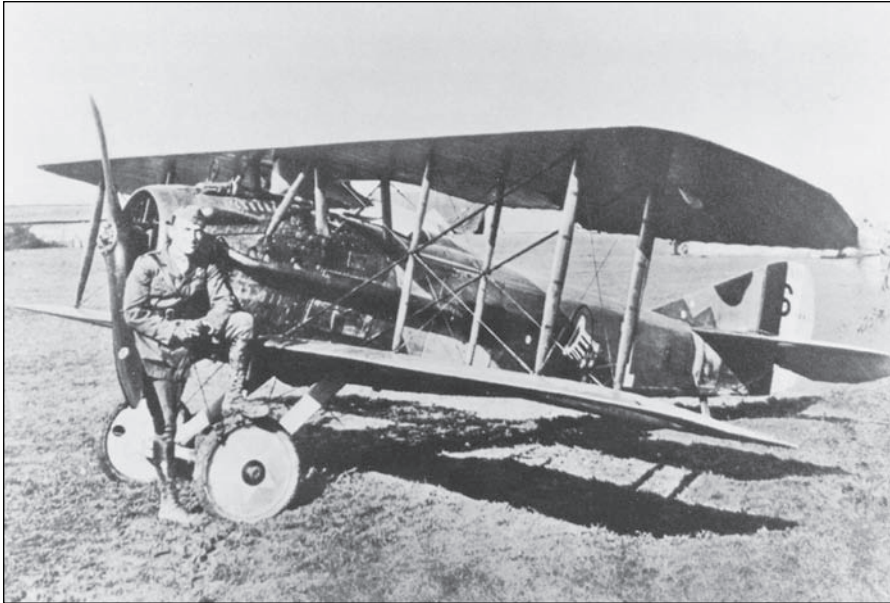
Figure 6.83 The French SPAD XIII, an example of the strut-and-wire biplane period. Captain Eddie Rickenbacker is shown at the front of the airplane. (Source: U.S. Air Force. )
