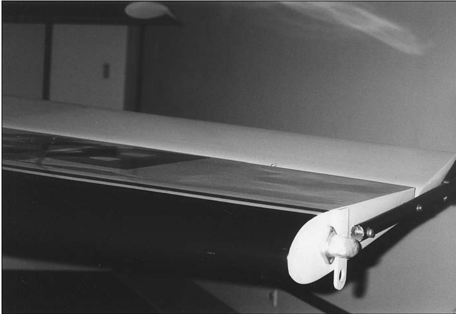
Figure 5.84 (concluded) (c) Detail of the left wing tip, showing the symmetric airfoil section.
