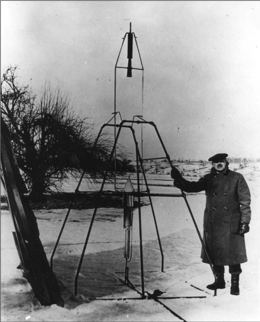
Figure 9.39 Robert H. Goddard and his first successful liquid-fuel rocket. This rocket made the world's first successful flight on March 16, 1926. (Source: NASA.)
