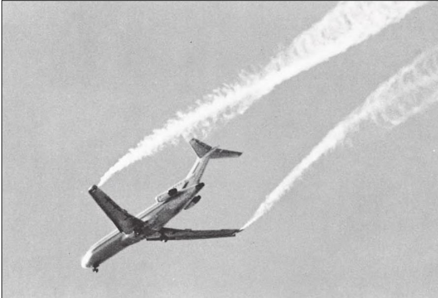
Figure 5.44 Wing-tip vortices made visible by smoke ejected at the wing tips of a Boeing 727 test airplane. (Source: NASA.)
