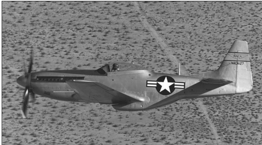
Figure 4.46 The first airplane to incorporate a laminar flow airfoil for the wing section, the North American P-51 Mustang. Shown is a late-model Mustang, the P-51D. (Source: Jim Ross/NASA. )
