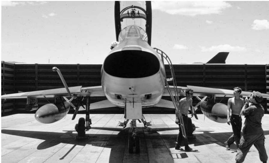
Figure 4.23 A North American F-100 from the 1950s. The Pitot tube extending ahead of the right wing leading edge is easily visible.
