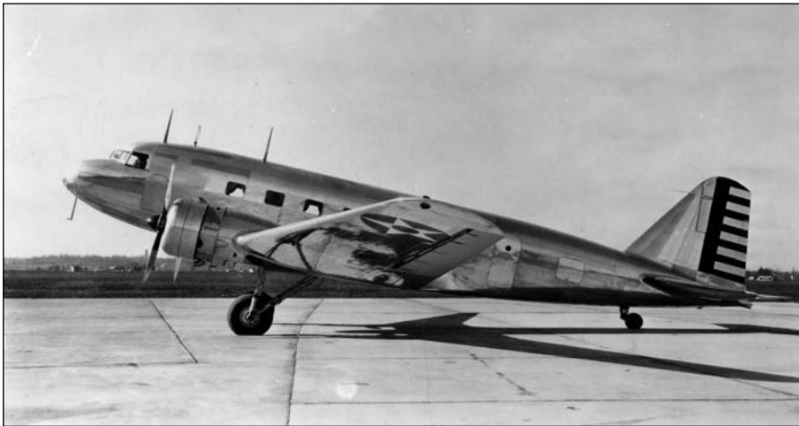
Figure 6.84 The Douglas DC-3, an example of the period of mature propeller-driven monoplanes with the NACA cowling and wing fillets. (Source: U.S. Air Force. )
