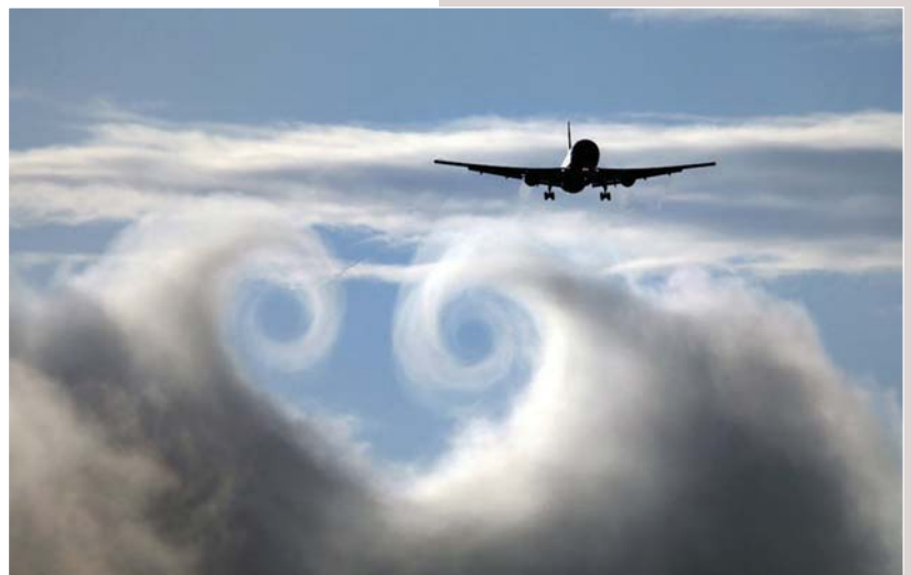
The wake of a Boeing 767 disrupts the top of a cumulus cloud and clearly shows the counter-rotating trailing vortices.
