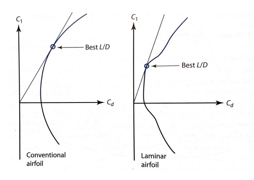
Airfoil design lift coefficient is the CI for maximum L/D
