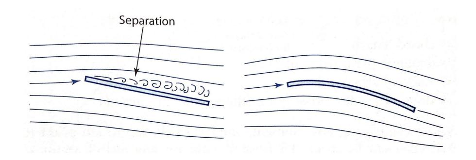
A flat plate will generate lift, but the flow will separate at moderate angles
