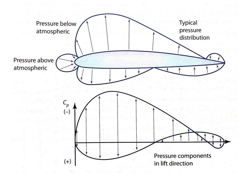
About 2/3 of the lift is produced by negative pressures over the top of the airfoil. So, if design features are to disturb a wing, it better be the bottom of it!
