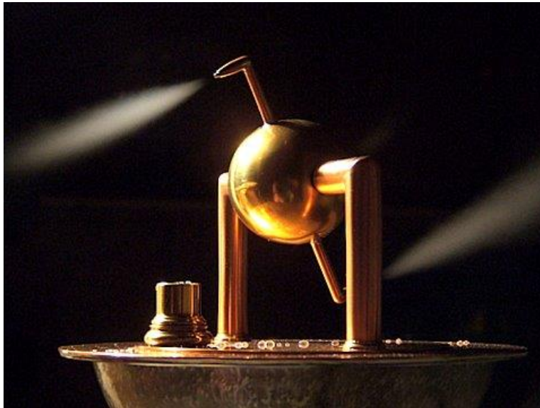
Figure 1.4 An Aeolipile, "the ball of Aeolus" is the first recorded steam engine or reaction steam turbine. Source: https://modelengines.info/aeolipile/
