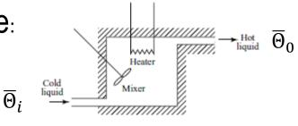
$\overline{\Theta}_i$ := steady-state temperature of inflowing liquid, °C  $\overline{\Theta}_0$ := steady-state temperature of outflowing liquid, °C G:= steady-state liquid flow rate,  $\frac{kg}{sec}$  M:= mass of liquid in the tank, kg c:= specific heat of liquid,  $\frac{kcal}{kg}$  °C R:= thermal resistance, °C sec/kcal C:= thermal capacitance,  $\frac{kcal}{c}$  $\overline{H}$ := steady-state heat input rate,  $\frac{kcal}{sec}$
