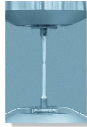
Typical necking pattern which has occurred on this steel specimen just before fracture.
