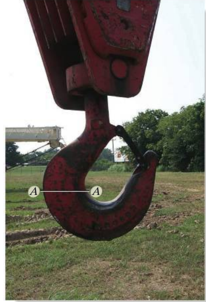
This crane hook represents a typical example of a curved beam.
