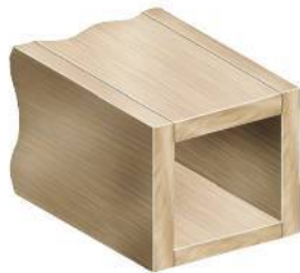
Wooden box beam
