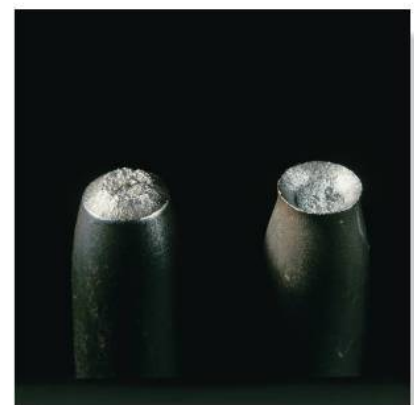
This steel specimen clearly shows the necking that occurred just before the specimen failed. This resulted in the formation of a "cup-cone" shape at the fracture location, which is characteristic of ductile materials.
