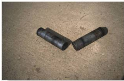
This pin was made from a hardened steel alloy, that is, one having a high carbon content. It failed due to brittle fracture.
