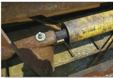
The drill shaft is connected to the soil auger using a shaft having a square cross section.
