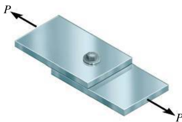
The area of the bolt for this lap joint is determined from the shear stress which is largest between the plates.
