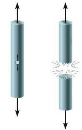
Failure of a brittle material in tension
