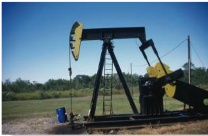
Engineers must account for possible fatigue failure of the moving parts of this oil-pumping rig.
