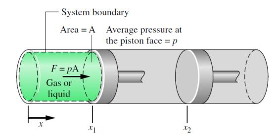
• For a change in volume from  $V_1$  to  $V_2$ , the work is obtained by integrating:
