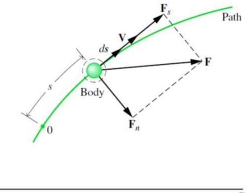
By Newton's second law of motion, the magnitude of the component F<sub>S</sub> is related to the change in the magnitude of V by:
