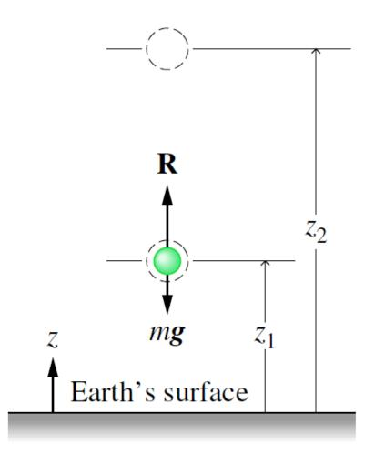
• The quantity mgz is the gravitational potential energy, PE. The change in gravitational potential energy,  $\Delta PE$ , is:
