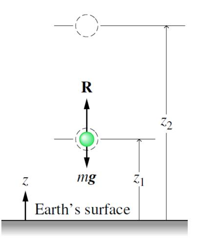
• The work of each force acting on the body shown in Figure can be determined by using the definition previously given. The total work is the algebraic sum of these individual values. The total work equals the change in kinetic energy. That is:
