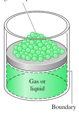
• For such idealized processes, the pressure *p* in the equation is the pressure of the entire quantity of gas undergoing the process and not just the pressure at the moving boundary.
