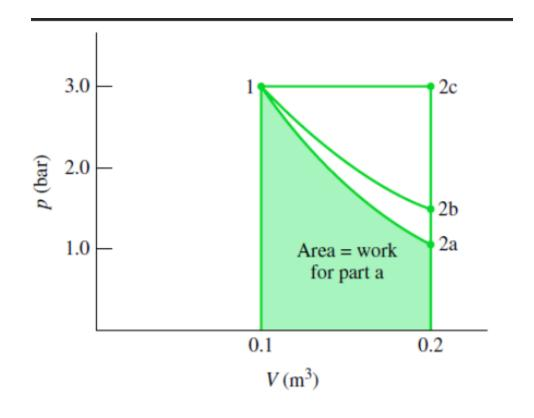
(a) Introducing the relationship  $p = constant/V^n$  into Eqn. 14 and performing the integration:
