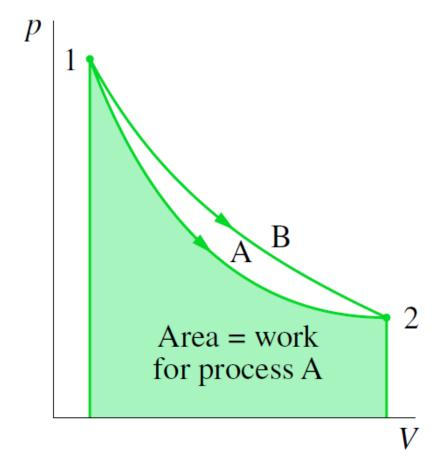
• The relationship between pressure and volume during an expansion or compression process also can be described analytically. An example is provided by the expression  $pV^n = constant$ , where the value of n is a constant for the process. A quasi-equilibrium process described by such an expression is called a polytropic process. Additional analytical forms for the pressure-volume relationship also may be considered.
