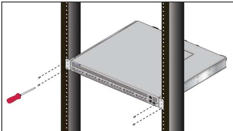
**Figure 3-6: Inserting the Switch into the Rack**
