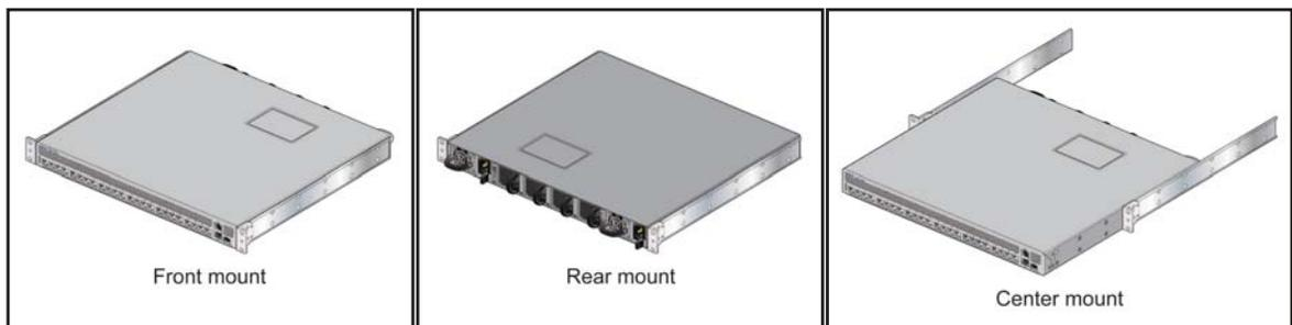
Figure 3-3: Bracket Mount Examples for Two-Post Rack Mount
