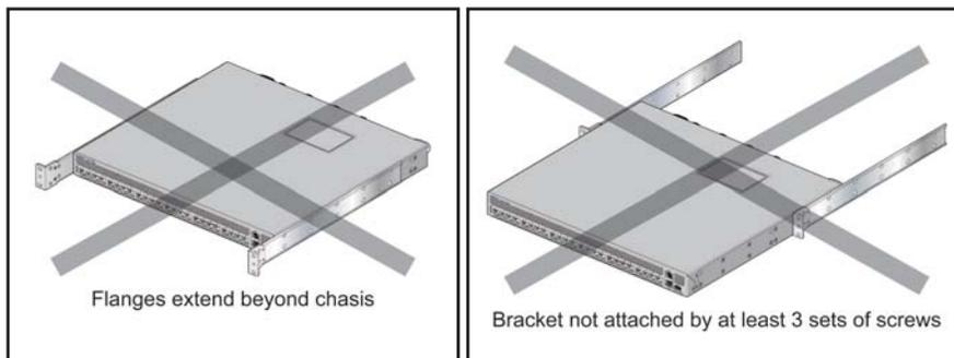
Figure 3-4: Improper Bracket Mount Examples for Two-Post Rack Mount
