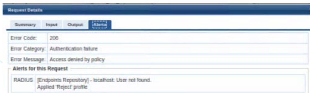
Figure 22. Unsuccessful Authentication in ClearPass Access Tracker
