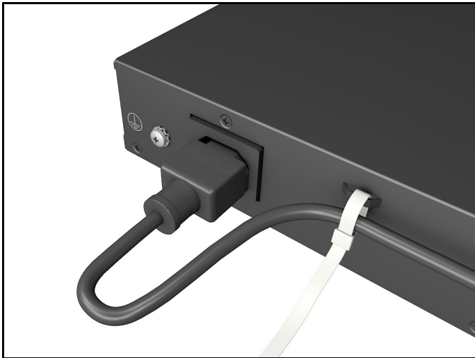
Figure 12 Using the cable tie on the 2540 switches
