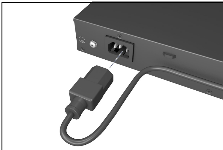
Figure 5 Connecting the power cord on the Aruba 2540 switches
