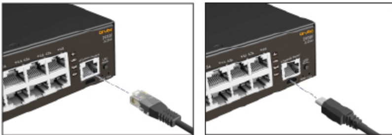
Figure 21: Connecting a console cable
