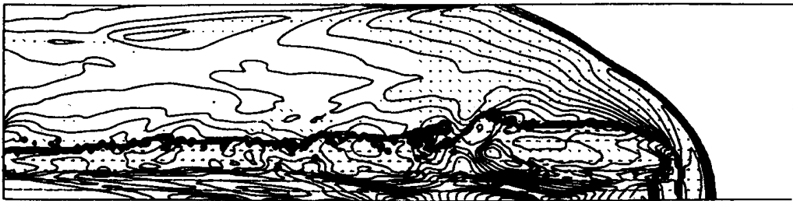
Fig. 8.13. A numerical simulation of a jet with a Mach number equal to 6. Contours represent lines of constant projected density. At each point of the grid the direction and modulus of the velocity are represented by a short segment. Oblique shocks along the jet as well as Kelvin-Helmholtz surface instabilities can be seen. (From Norman et al. 1982)
