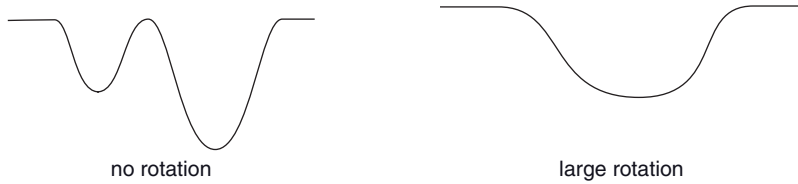
Figure 4.8 Illustration of the blending of two atomic lines. On the left, two atomic lines are shown in a spectrum of a star that does not rotate, while on the right, these two lines are blended together for a star with a large rotational velocity. Note that the blended line is no longer symmetric.
