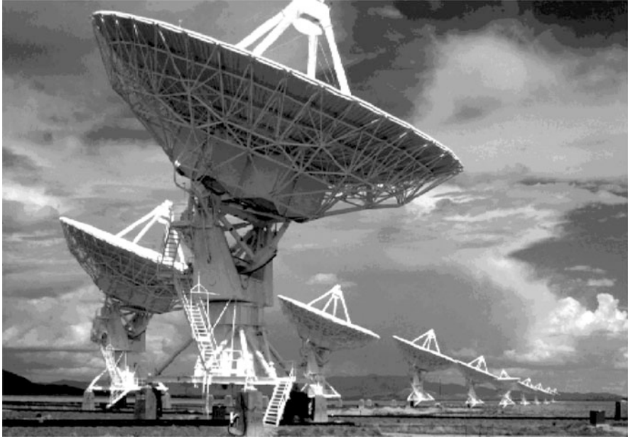
Fig. 4.3 The Very Large Array (VLA) is a collection of 27 radio antennas located at the NRAO site in Socorro, New Mexico. Each antenna in the array measures 25 meters (82 feet) in diameter and weighs about 230 tons. The VLA is an interferometer, which means that the data from each antenna can be combined electronically so that the array effectively functions as one giant antenna. Credit: NRAO/AUI/NSF
