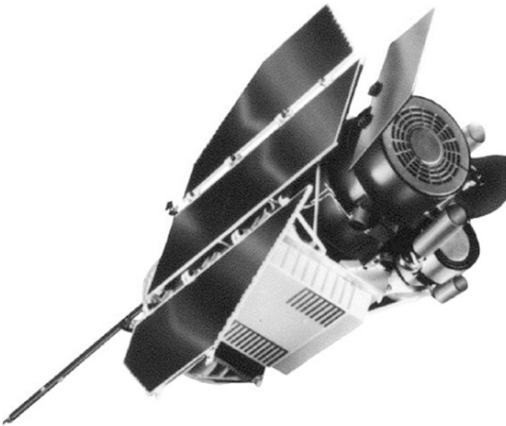
Fig. 2.9 Model of ROSAT in flight configuration. Throughout the 1990s ROSAT observed major star-forming regions in X-rays. One of its major accomplishments was the completion of the first X-ray all-sky survey (RASS). Credit: Max Planck Institut für extraterrestrische Physik
