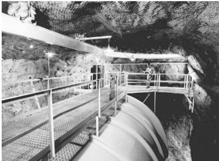
FIGURE 11.8 Raymond Davis's solar neutrino detector. The tank was located 1478 m (4850 ft) below ground in the Homestake Gold Mine in Lead, South Dakota, and was filled with 615,000 kg of C_2Cl_4 in a volume of 377,000 liters (100,000 gallons). (Courtesy of Brookhaven National Laboratory.)
