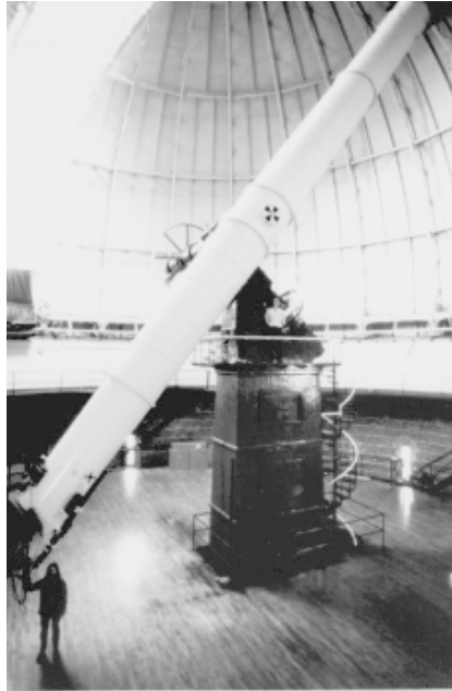
FIGURE 6.16 The 40-in (1.02-m) telescope at Yerkes Observatory was built in 1897 and is the largest refractor in the world. (Courtesy of Yerkes Observatory.)
