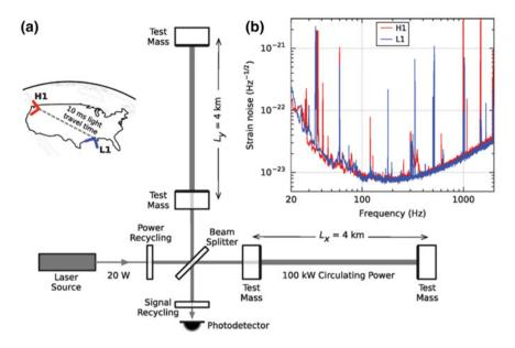
**Fig. 12.5** Sketch of the advanced LIGO detectors, location and orientation of the LIGO detectors at Hanford (H1) and Livingston (L1) (**a**), and sensitivity curves in terms of equivalent gravitational wave strain amplitude (**b**). From [1] under the terms of the Creative Commons Attribution 3.0 License
