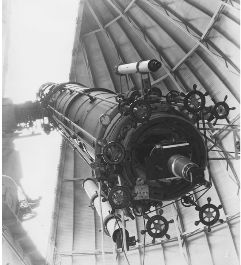
Fig. 3.11 The largest refractor in the world is at the Yerkes Observatory, University of Chicago. It has an objective lens with a diameter of 102 cm. (Photo by Yerkes Observatory)
