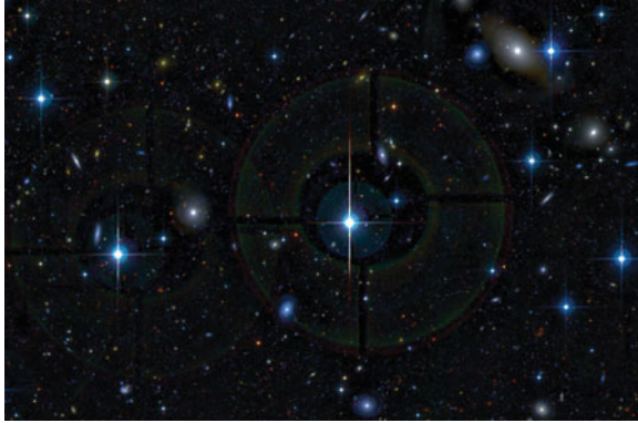
Fig. 9.12 Part of an image of a very deep field obtained with the MEGACAM camera at the focus of the Canada–France–Hawaii telescope. Note two types of artifacts around the bright stars. First, there are two extended and overlapping halos due to unwanted reflections on the lenses of the focal reducer. These are circular and reproduce an image of the telescope pupil with its central obstruction. Then there are spikes in the shape of a cross. These result from the diffraction of light on the arms of the spider which holds the mechanical structure in which the camera is installed at the primary focus
