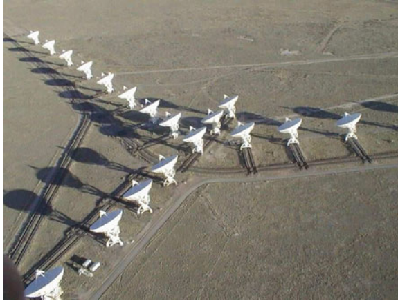
Fig. 6.35 Aerial view of the antennas of the VLA (Very Large Array) aperture synthesis array. The antennas are arranged in the shape of a Y, with the northern branch on the right, the south-eastern branch on the left, and the south-western branch at the top. Each branch includes 24 possible antenna positions at which the 27 mobile antennas can be placed. (NRAO photograph, Associated Universities, with the kind permission of the National Science Foundation)
