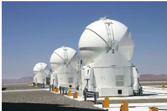
Fig. 6.46 Three of the mobile 1.8 m telescopes of the VLTI, which is the interferometric configuration of the Paranal VLT. Original photo with the courtesy of Pierre Kervella
