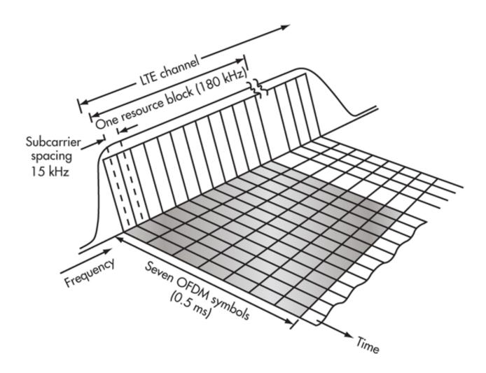
5. OFDMA assigns a group of subcarriers to each user. The subcarriers are part of the large number of subcarriers used to implement OFDM for LTE. The data may be voice, video, or something else, and it's assembled into time segments that are then transmitted over some of the assigned subcarriers.
