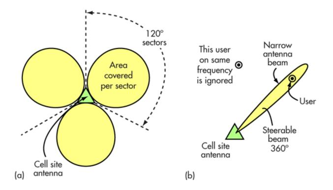
6. SDMA separates users on shared frequencies by isolating them with directional antennas. Most cell sites have three antenna arrays to separate their coverage into isolated 120° sectors (a). Adaptive arrays use beamforming to pinpoint desired users while ignoring any others on the same frequency (b).
