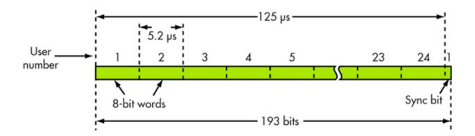
2. This T1 digital telephony frame illustrates TDM and TDMA. Each time slot is allocated to one user. The high data rate makes the user unaware of the lack of simultaneity.
