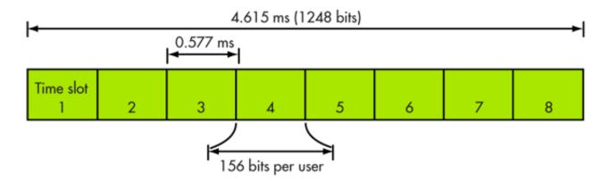
3. This GSM digital cellular method shows how up to eight users can share a 200-kHz channel in different time slots within a frame of 1248 bits.
