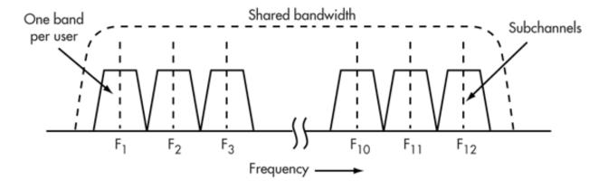
1. FDMA divides the shared medium bandwidth into individual channels. Subcarriers modulated by the information to be transmitted occupy each subchannel.
