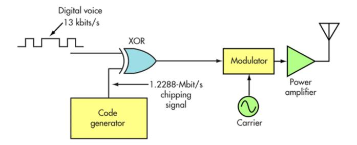
4. Spread spectrum is the technique of CDMA. The compressed and digitized voice signal is processed in an XOR logic circuit along with a higher-frequency coded chipping signal. The result is that the digital voice is spread over a much wider bandwidth that can be shared with other users using different codes.
