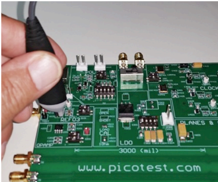
24-4. Picotest's 1-Port probe is used to make an output impedance measurement of a voltage reference.
