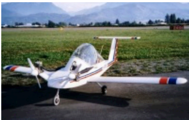
23-5. Cri-Cri uses composite materials instead of metal to reduce overall weight and make room for the high-energy-density lithium batteries that provide power to four brushless electric motors—two mounted back-to-back on nose pods on each side—with counter-rotating propellers.
