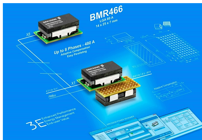
4-5. The BMR466's unique LGA (Line Grid Array) footprint is 0.98 × 0.55 in. and has an exceptionally low profile of 0.276 in., which facilitates compact system design.
