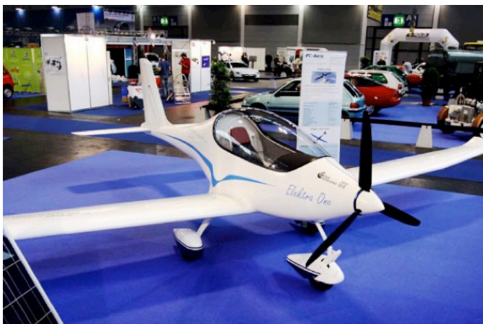
23-4. Elektra One has a maximum power of 16-20 kW, and range is more than 400 km (249 miles) with a flight time of up to more than three hours.
