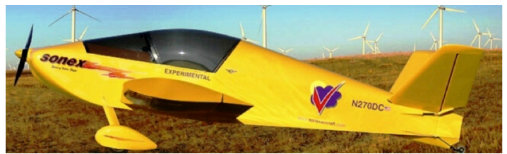
23-7. The Sonex electric airplane will use a dc cobalt motor, controller, and highly efficient battery and charging system. It will emphasize power-plant research and development.
