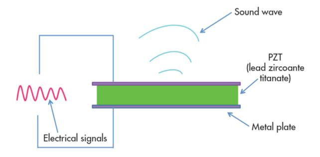
ng the inverse piezoelectric effect can help develop devices that generate and produce acoustic sound waves. Imples of piezoelectric acoustic devices are speakers (commonly found in handheld devices) or buzzers. The advantage of having such speakers is that they are very thin, which makes them useful in a range of phones. Even medical ultrasound and sonar transducers use reverse piezoelectric effect. Non-acoustic inverse piezoelectric devices include motors and actuators.
