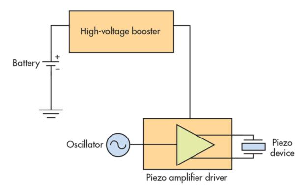
*Figure 5* is a block diagram that illustrates piezo-driver operation. Piezo drivers will take low battery voltage and use a booster to convert it to higher voltage. The higher voltage is then used to power the amplifier. The oscillator will input small sine waves, which the amplifier will change into larger voltage sine waves. The amplifier drives the piezo device.
