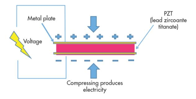
Piezoceramic material—non-conductive piezoelectric ceramic or crystal—is placed between the two metal plates. For piezoelectricity to be generated, it needs that material to be compressed or squeezed. Mechanical stress applied to piezoelectric ceramic material generates electricity.
