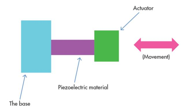
The piezoelectric actuator has many uses and applications. For example, knitting machinery and braille machines use these actuators, since they have such a small amount of moving parts and a very simple design. They can even be found in video cameras and cellular phones, because they are proven most proficient as an auto-focusing mechanism.<sup>10</sup>
