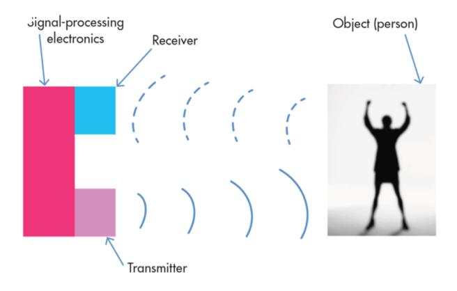
In Figure 3, sonar is sending out, via transmitter, a sound wave (signal) to search for objects ahead. The transmitter uses inverse piezoelectric effect, which is when the transmitter will use voltage to help it send out a sound wave. Once the sound wave hits an object, it will bounce back. The sound wave that bounces back will be detected by the receiver.
