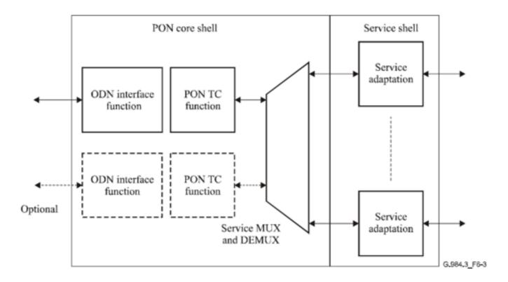
Functional blocks are similar to the OLT. In the scenario that the ONU/OLT operates with a single PON interface (max 2 for protection purposes) the cross-connect function is omitted. Instead of this function, the service MUX and DEMUX are now responsible for traffic.
