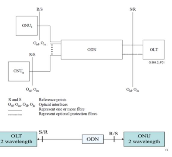
• The OLT is connected to the optical splitter through a single optical fiber, and then the optical splitter connects to ONUs/ONTs.
