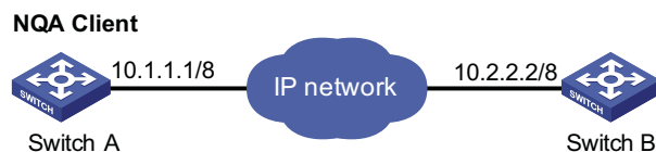
Figure 309 Network diagram for the ICMP-echo test
