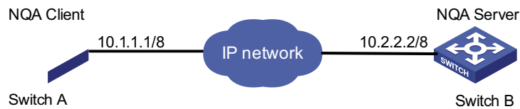
Figure 313 Network diagram for UDP-jitter test
