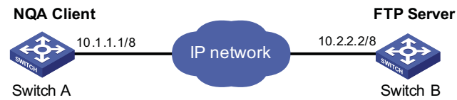
Figure 311 Network diagram for FTP
