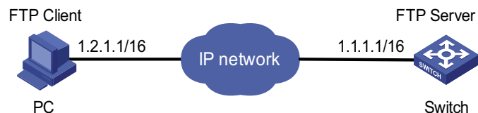
Figure 299 Smooth upgrading using the FTP server
