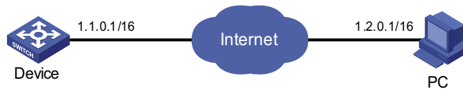
Figure 303 Network diagram for outputting log information to a Linux log host
