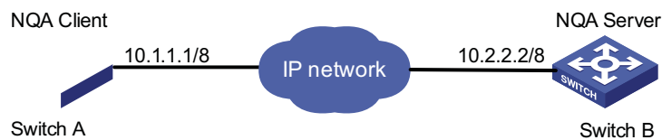
Figure 315 Network diagram for the TCP test
