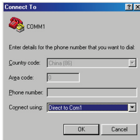
Figure 5 Specify the port used to establish the connection
