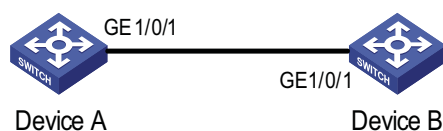
Figure 28 Network diagram for port-based VLAN configuration
