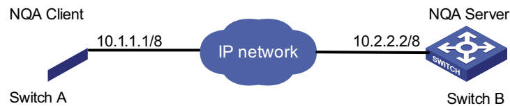
Figure 316 Network diagram for the UDP-echo test
