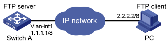
Figure 1-1 Network diagram for configuring a switch as FTP server
