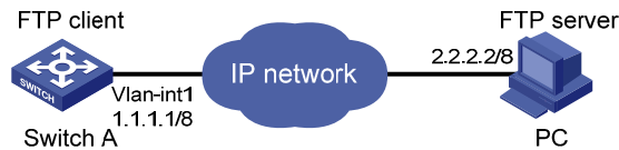
Figure 1-2 Network diagram for configuring a switch as FTP client
