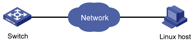
Figure 1-2 Network diagram for outputting log information to a Linux log host
