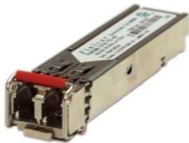
Figure 5 Appearance of a Gigabit CWDM transceiver module
