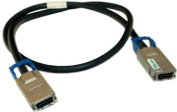
Figure 11 Appearance of a CX4 cable
