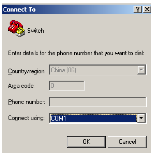
Figure 119 Specifying the connection port
