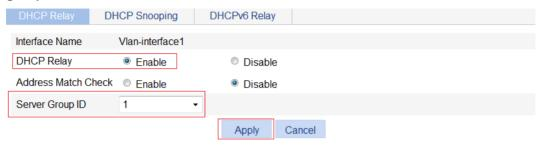
Because the DHCP relay agent and server are on different subnets, you need to configure a static route or dynamic routing protocol to make them reachable to each other.
