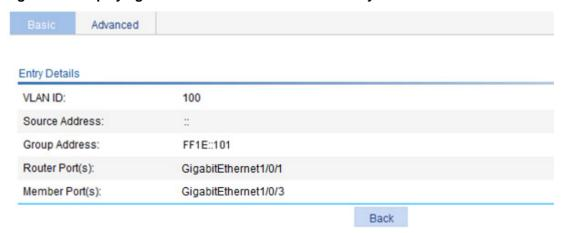
The output shows that GigabitEthernet 1/0/3 of Switch A is listening to multicast streams destined for IPv6 multicast group **FF1E::101**.
