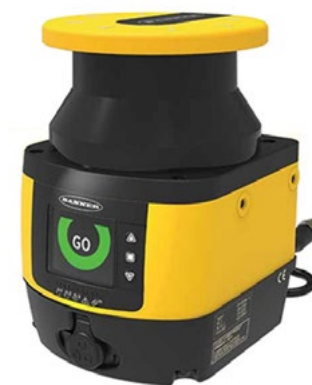
Figure 2: The Banner Engineering SX5-B safety laser scanner has a maximum range for safety and warning zones of 5.5 m and 40 m, respectively. It can provide 275 degrees of coverage and is immune to ambient light and dust. (Image source: Banner Engineering)
