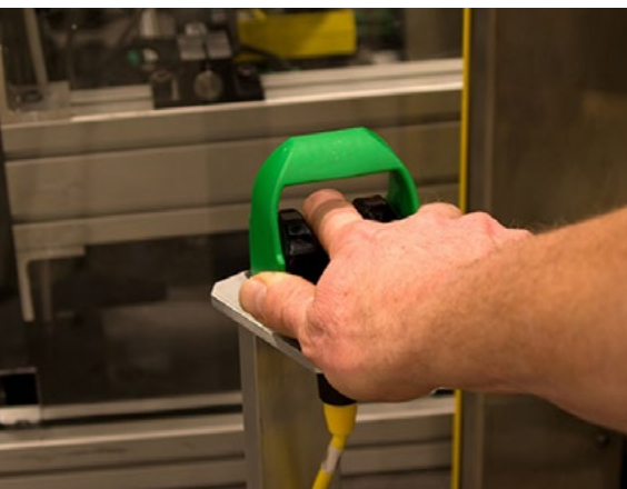
Figure 3: The mere closing of guard interlocks doesn't trigger the restart hazardous machine processes; instead, those honors go to a separate double-duty control interlock or start switch like the soft-touch capacitive finger switch shown here. (Image source: Getty Images)
