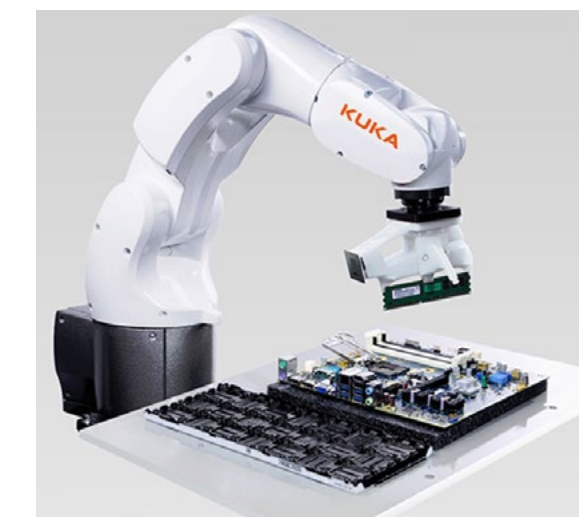
Figure 6: Compact industrial robots such as the KUKA Agilus KR 3 are designed with safety as a major consideration and can safely share workspace and collaborate with human operators if industry standards are followed during setup. (Image source: Kuka Robotics)
