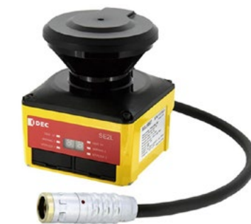
Figure 3: The IDEC SE2L-H05LPC safety laser scanner supports a 270-degree protection field for up to 5 m. Four SE2L scanners can be easily connected together using RS-485 for simultaneous operation. (Image source: IDEC)
