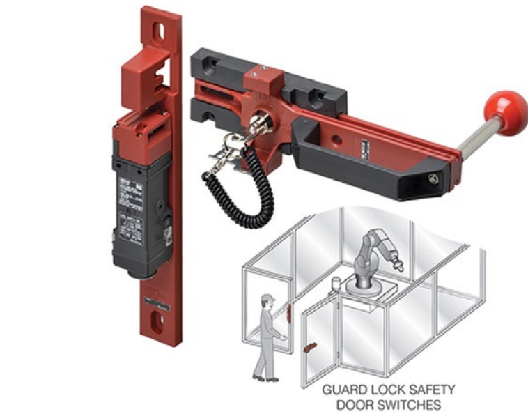
Figure 4: Some doubly capable interlocks have actuators to function as guard locks. These are position switches with deadbolts or electromagnetic assemblies that can keep doors barred until the guarded robotic arm or machine ceases its hazardous motion. Unfortunately, some engineers mistakenly believe that all interlocks are of the guard-lock variety. (Image source: Omron )
