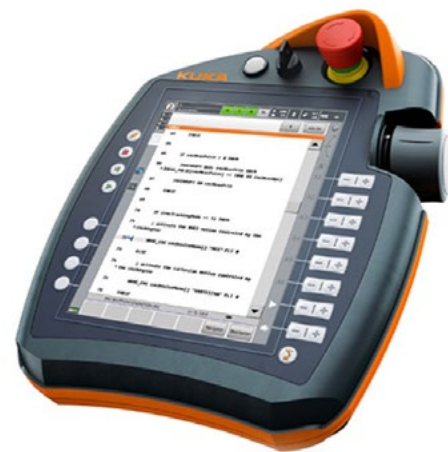
Figure 7: The KUKA robot kits include a smartPad touch operator panel to enable hand-guided control where appropriate. (Image source: KUKA Robotics)
