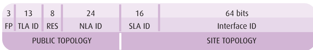
IPv6 Aggregatable Global Unicast Address Format
