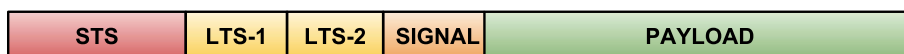
Fig. 3 WiFi frame structure: LTS-1 and LTS-2 are used for channel and noise variance estimation
