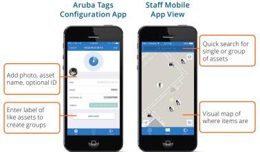
The data can also be used as an inventory list, for PAR-level management and to indicate the status of an item (e.g., available, being cleaned, etc.). The Aruba Tags are easily moved from one asset to another and relabeled using the Aruba Asset Tracking Configuration app.
