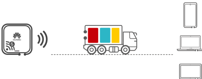
Figure 3-2 Multi-user transmission in Wi-Fi 6
