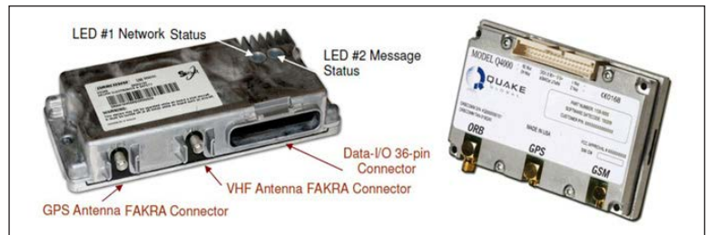
▲ Fig. 7 ORBCOMM second generation of SCU modems: Stellar DS300 (a) and Quake Q4000 (b). 11,12
