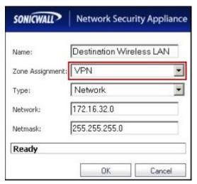
Group to be created in Site A SonicWALL with Destination LAN and WLAN **Network Security Appliance** SONICWALL Destination Network 12daf1 g VAP BSSID 1 12daf1 Radio a BSSID Destination LAN Destination Wireless LAN 12daf1 Radio g BSSID 192 168 10 100 192.168.160.130 Default Active WAN IP Default Gateway Destination Dial-Up Default Gateway face Ready OK Cancel
